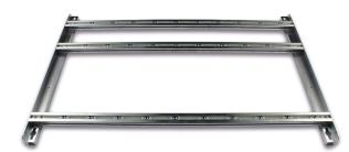
Support frame for 912-series headends with redundant power supplies. It can hold up to 2 power supplies, one amplifier and 7 modules, or 2 power supplies and 8 modules. There is a 47 mm distance between modules to allow for better heat disipation.
