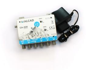
Head-end broadband amplifier with three inputs and two outputs. It has two UHF inputs and another input for BI/FM/BIII/DAB. The two outputs have the same output level, with a maximum of 110 dB $\mu$ V, and facilitate the creation of star-shaped distributions using splitters.
