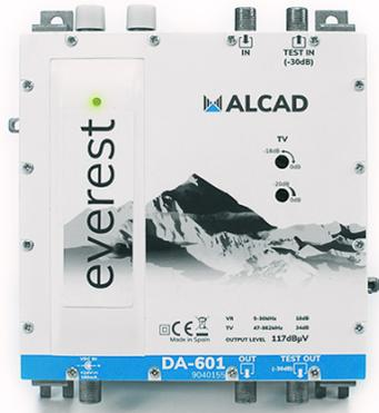
Broadband distribution amplifier for terrestrial TV (117 dBuV). It has a gain control and variable slope control. It amplifies the return path from 5 to 30 MHz. Fed by an external power supply model FF-200 (included with the amplifier). The input and output test points permit checking and adjusting the installation with no need to disconnect the TV signal.
