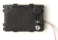
Module with loudspeaker and microphone for entrance panel. It has a voice synthesizer in 14 languages for the "Open door" message. It has an 8 ohm speaker with plastic membrane to prevent deterioration over time in outdoor conditions. (Compatible with GRF-302 and GRF-304 version 10F or higher, it is essential to raise switch n°4 of the GRF to activate the spoken message)
