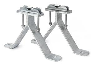
Stand Off Wall Mast Mount, Y-Type, Height = 190 mm, Thickness = 5 mm; Hot-dip galvanized Steel. MoQ = 2 units. Screws M10. For mast  $\emptyset$  30 to 60 mm.
