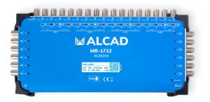
Final multiswitches for 16 polarities and terrestrial TV with 12 outputs. The outputs are amplified in the satellite IF band. Need to be powered from each individual receiver so that the switching and the amplification of each derived output will function correctly. The external power supply units provides the required voltage to the LNBs in order to work properly.
